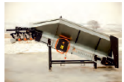
Bunker with adjustable separator
