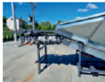
Bunker with a permanent separator
